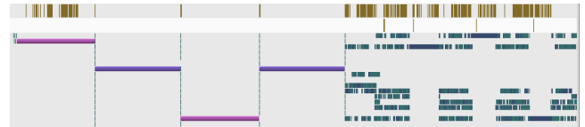
Figure 8: A profiler snapshot of 5 concurrent IO kernels reading from disk with preemptive IO and the compute kernels. Long lines are compute kernels. Note that the horizontal axis scales here and in Figure 7 are different, but the actual kernel execution time is the same.
